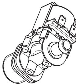
2) Fixing possibility for self tapping screw  $\varnothing$  3,5
