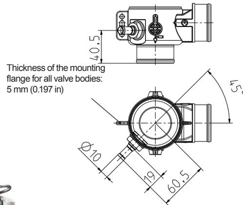
Thickness of the mounting flange for all valve bodies: 5 mm (0.197 in)
