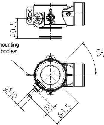
Thickness of the mounting flange for all valve bodies: 5 mm (0.197 in)
