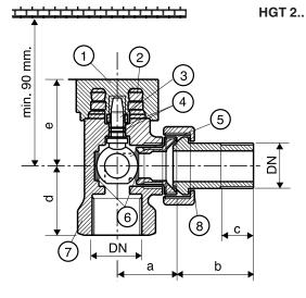
1 – Knob 2 – Lugs for coupling to actuator
