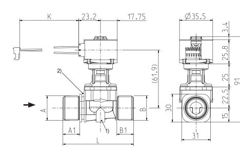
1) Fixing possibility for self tapping screw Ø 4,2 2) Fixing groove
