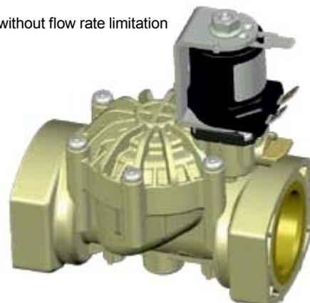
The flow rate can be limited by turning the slotted screw in the valves cover cone.
